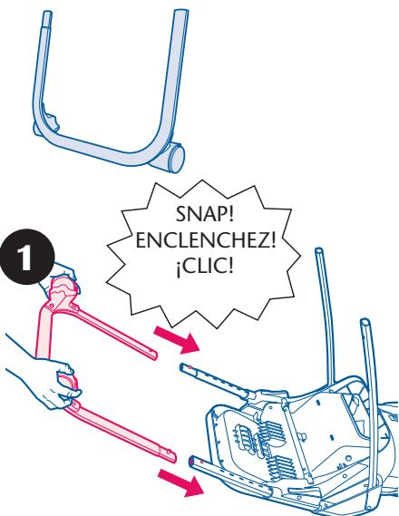
Insert "U" tube with wheels into the front leg tubes.
